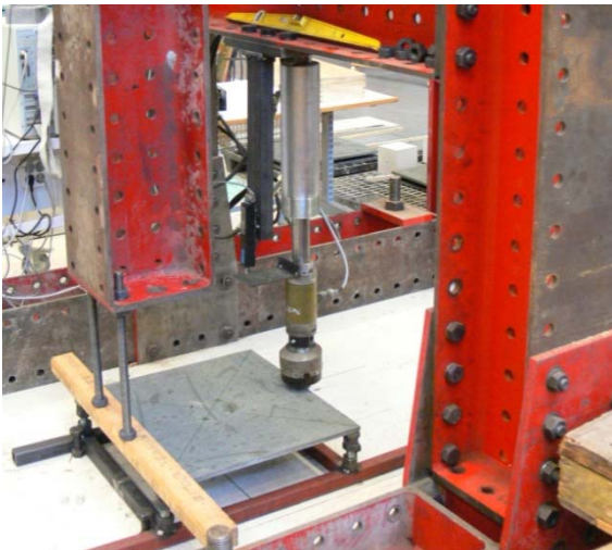
Figure 6: The testing machine with a thin plate placed on four supports; the loading head is placed between two supports at the edge of the plate.
