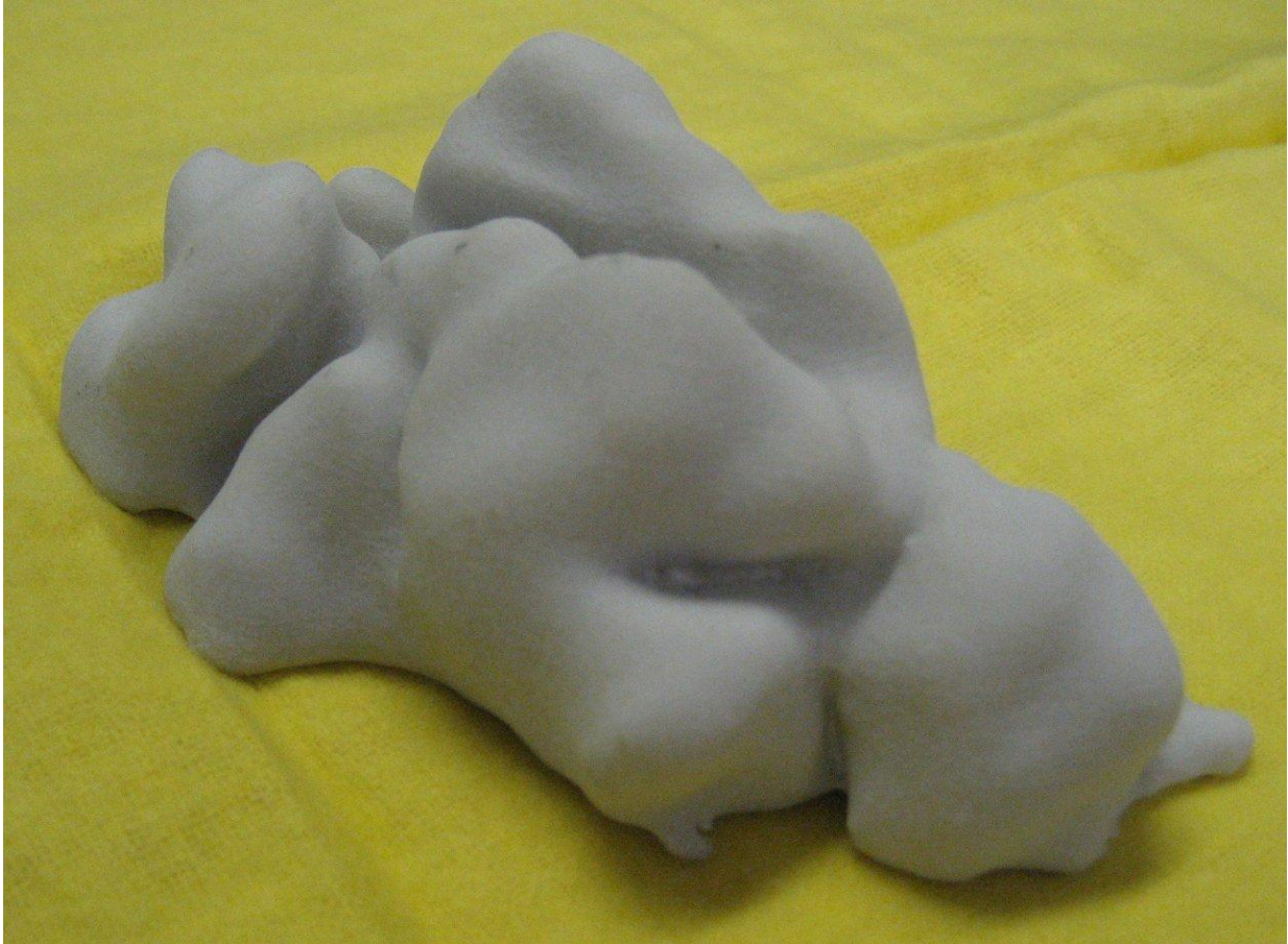
Figure 1. Rapid Prototype reconstruction of a segment of a turbulent flame
