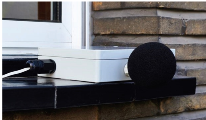
Figure 3 – Example of a sensor node, placed on the windowsill of a dwelling.
