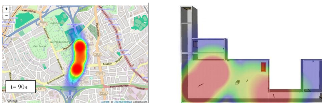
Figure 2: Mapping of smoke risk level on OpenStreetMap (left) and on building information map (right)
