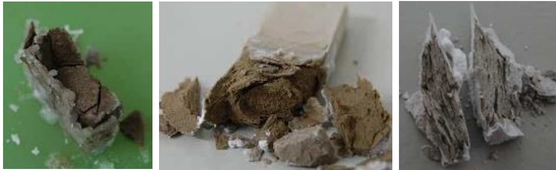
Fig.2 Visual observation of CSA cement paste specimen exposed to 10% Na 2 SO 4 solution
