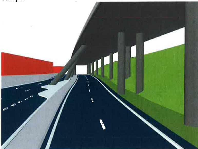
Fig. 3: Visualisation of the piers underneath the viaduct
