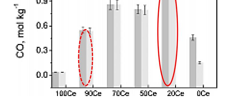
In order to understand the structural interaction, a series of  $Fe_2O_3$  was prepared and investigated using in situ XRD and XAS at 700°C in chemical looping process. The most active material (80%  $Fe_2O_3$ -CeO<sub>2</sub>) from our previous study [1] and the material with a low amount of incorporated Fe (10%  $Fe_2O_3$ -CeO<sub>2</sub>) as seen from the change in lattice parameters, have been pursued for this investigation.
