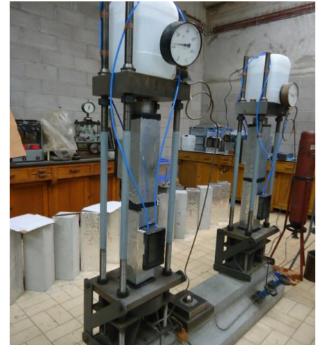
Figure 2. Chloride and load combined attack setup (compression)
