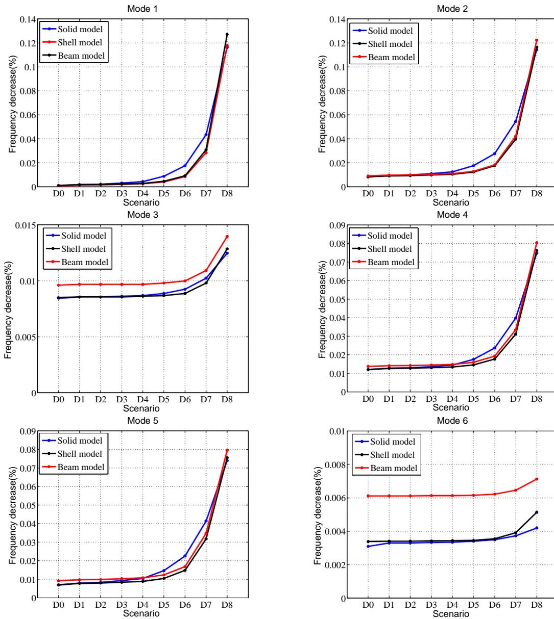
**Figure 8.** Natural frequency change of mode one to six for the three models.
