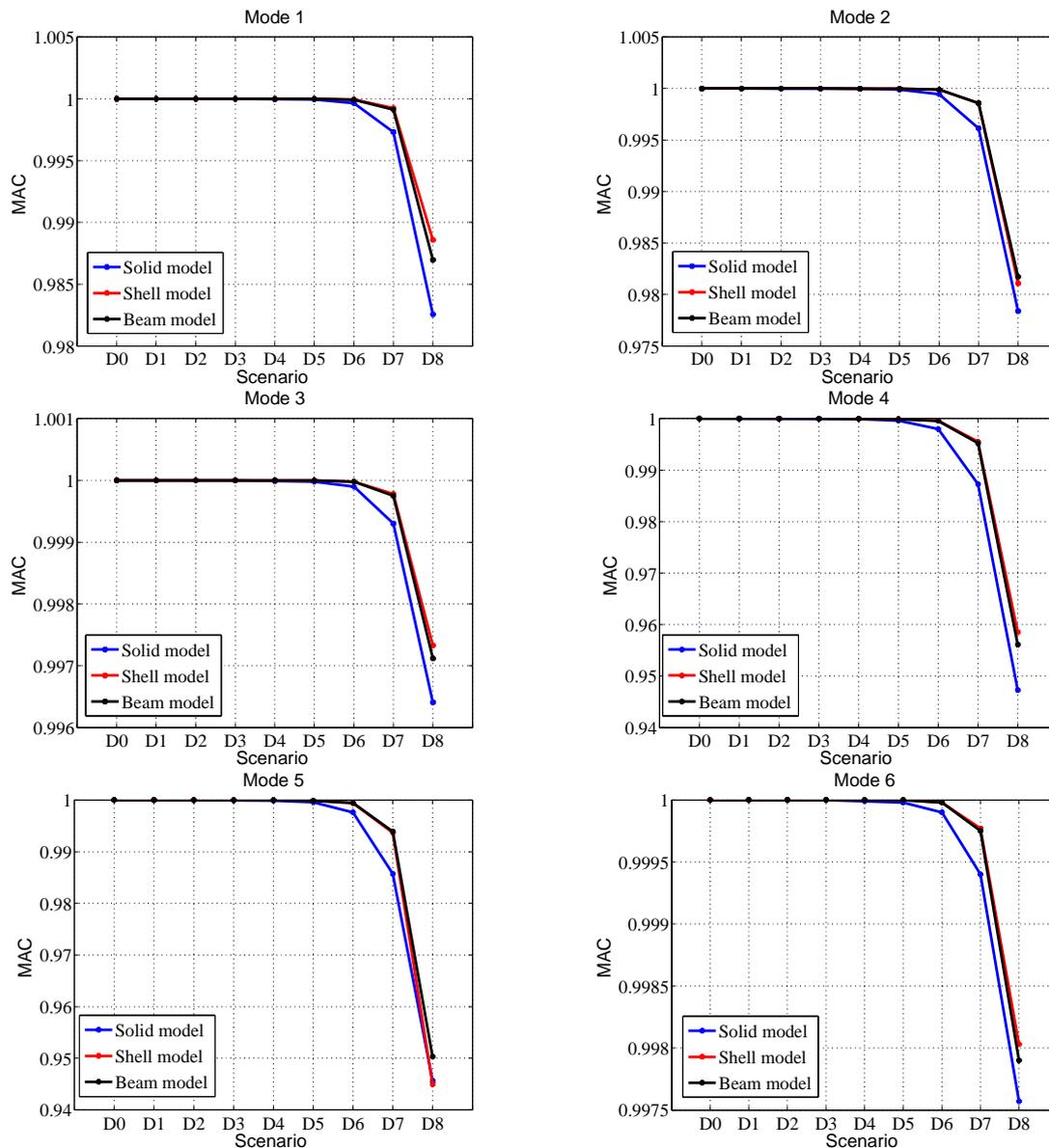
**Figure 9.** MAC value of mode shape from mode one to six for the three models.
