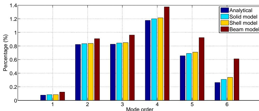
**Figure 7.** Frequency difference to the experimental value.
