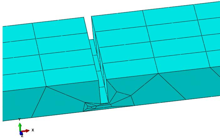
**Figure 4.** Zooming saw cut with solid model.
