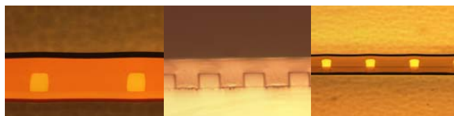
Figure 2 Complete stack with photolithographic waveguides in left : Ormocor®, middle : Epocore (on FR4-material) and right : Truemode™
