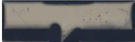
Figure 6: Micro-optical out-of-plane coupler.
