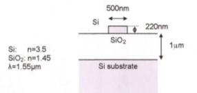
Because of the limited thickness of the oxide buffer, some part of the power in the fundamental mode will leak to the substrate. The aim of this exercise was to calculate the complex propagation constant of the fundamental mode of this structure as accurately as possible.
