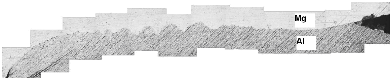
Figure 4: Microscopic image of a MPW over the entire length of the weld [4]
