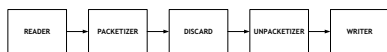
Figure 3. Configuration as impairment tool which drops parts of frames. The component discard drops the packets it receives with a given probability.
