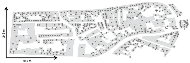
Fig. 2. Overview of the target area and the possible locations (squares) for femtocell base stations in the target area (0.11 km 2 ).
