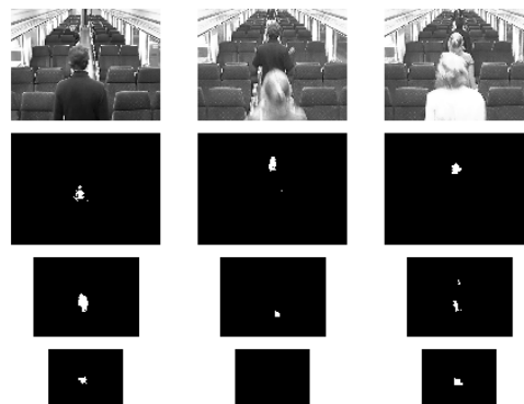
Figure 2: The input image at the largest scale and the results of the Adaboost classification at all three scales.
