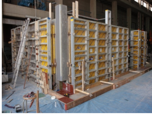
Figure 1: Layout of the formwork filling tests.
