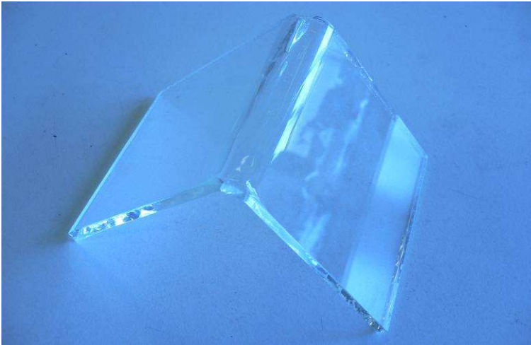
Figure 8: Sample with direct fused glass plates (i.e. without joint filler) on perpendicularly polished edges
