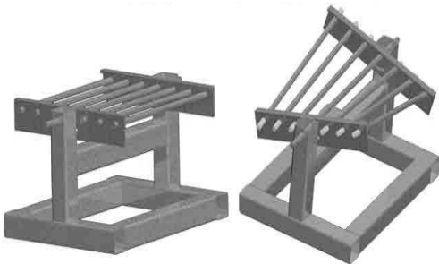
Figure 1: Schematic representation of preliminary adjustable moulds used for exploration of thermoforming parameters
