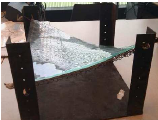
Figure 5: Double curved glass shell on “Sierra papa 2” stainless steel mesh
