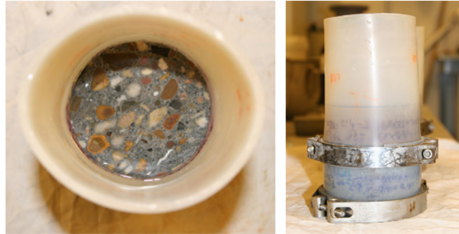
Figure 2: Specimen sealed with rubber sleeve and stainless steel clamps
