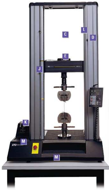
Figure 10: Instron 5543 for cyclic stretching of the embedded meandered copper tracks
