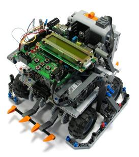
Fig. 3. A typical example of a robot build by the students. One can identify the microcontroller board, a set of motors, battery back and sensors.
