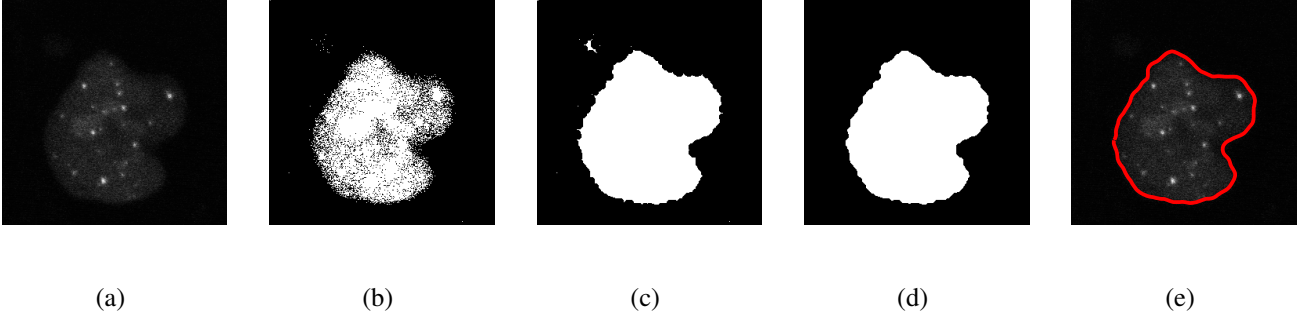
Figure 1: An example of the different steps in the segmentation algorithm. (a) shows the projection of the 3D micrograph on a 2D image. (b) demonstrates the result of Otsu thresholding. (c) and (d) are respectively the morphological opening and closing. (d) shows the filtered contour plotted on top of the image.
