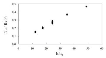
Figure 9. The dimensionless group Nu/RePr varies linearly with h/b0. Simulations of geometry B for  $\alpha_0 = 0$ .
