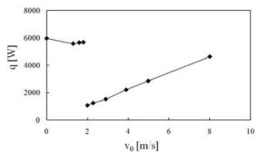
Figure 7. Heat transfer rate is a linear function of outlet velocity. Simulations of geometry B, door width w = 2 m.
