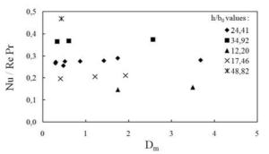
Figure 8. The dimensionless group Nu/RePr is independent of the deflection modulus. Simulations of geometry B for  $\alpha 0 = 0$ .
