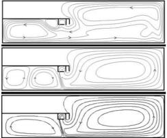
Figure 5. Streamline patterns (kg/s) for the 3 regimes: natural convection, mixed convection and forced convection. Simulations of geometry B.
