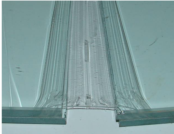
Figure 5: Detail of a particular final delamination pattern of a sample tested at 45°C
