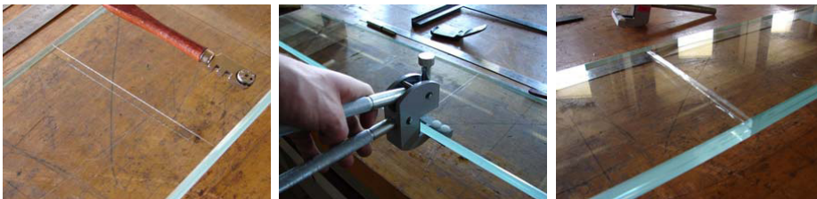
Figure 1: Making initial cracks : scratching the surface / cracking a glass plate / resulting initial cracks .
