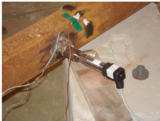
Figure 2: Pressure sensor, strain gauges and temperature sensor.
