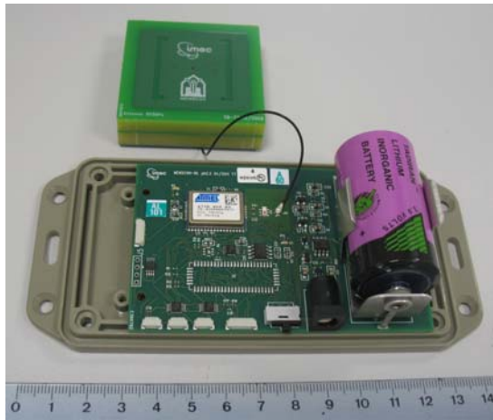
Fig. 5: Wireless sensor module inside opened housing ceiling using screws, and offering access for sporadic battery replacement if needed. The core components are:
