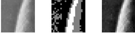
Fig. 4: Examples of neighbourhood transforms for an input neighbourhood (left). In the middle, the census transform results in either -1,0 or 1 depending on whether it has a lower value, a similar value or a higher value than the central pixel. To the right, the normalization transform subtracts the mean from each pixel and divides by the neighbourhood variance.
