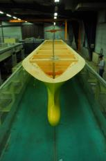
Figure 5: View of the Post-Panamax container ship model
