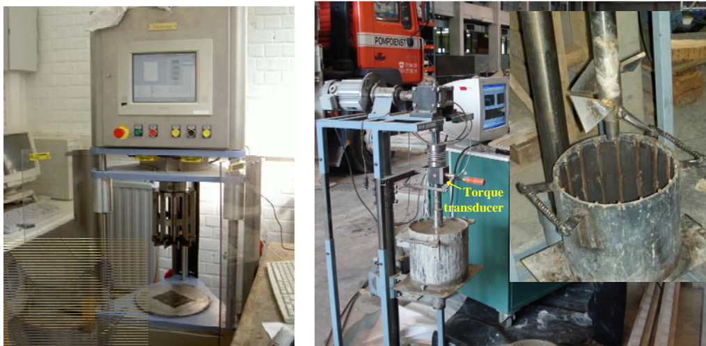
Figure 2. Left: ConTec Viscometer. Right: Tattersall Mk-II rheometer.
