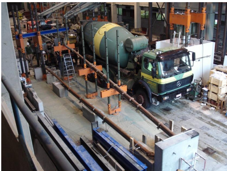
Figure 1. Short pumping circuit (25 m).
