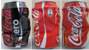
Figure 3: Failure pattern of empty cola cans
