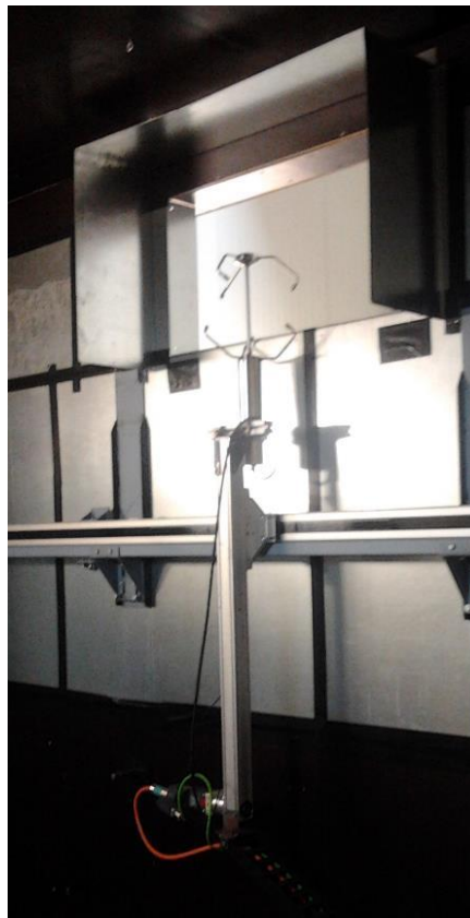
Fig. 4-6: Vent B with flange and 3D ultrasonic sensor mounted on the vertical guidance of the automated sensor frame.
