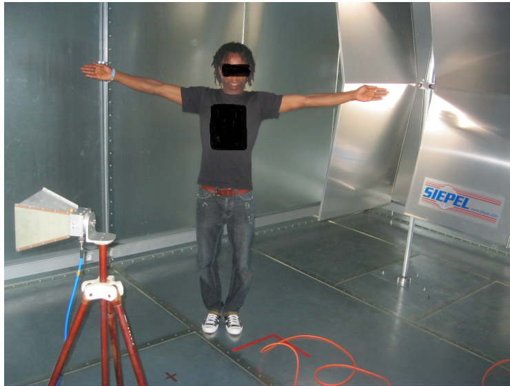
Figure 2.12: Human under test in the RC adopting the standing with stretched arms' posture
