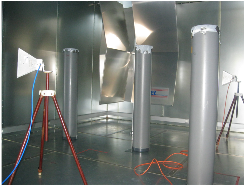
Figure 2.3: Phantoms and transceivers in the reverberation chamber. The RC dimensions are 2.80 m \times 5.70 m \times 4.10 m (Height \times Length \times Width)
