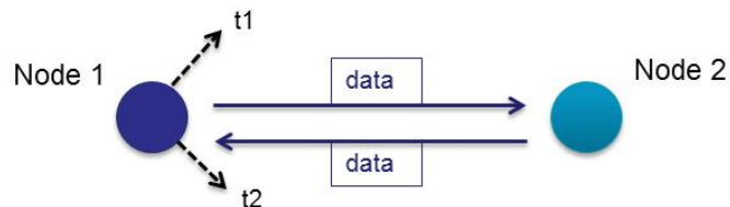
Figuur 9-5 Two Way Ranging
