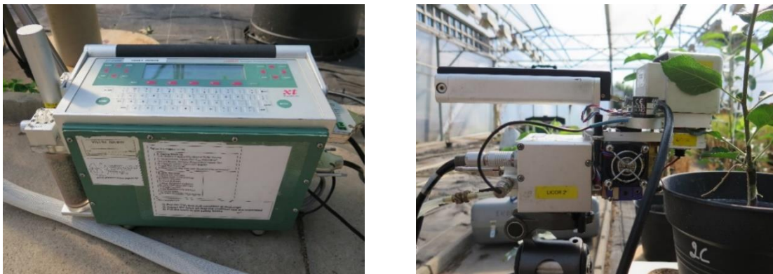
Figure 6-3. The Li-Cor LI-6400 Portable Photosynthesis System with Li-Cor 6400-40 Leaf Chamber Fluorometer as a sensor head.
