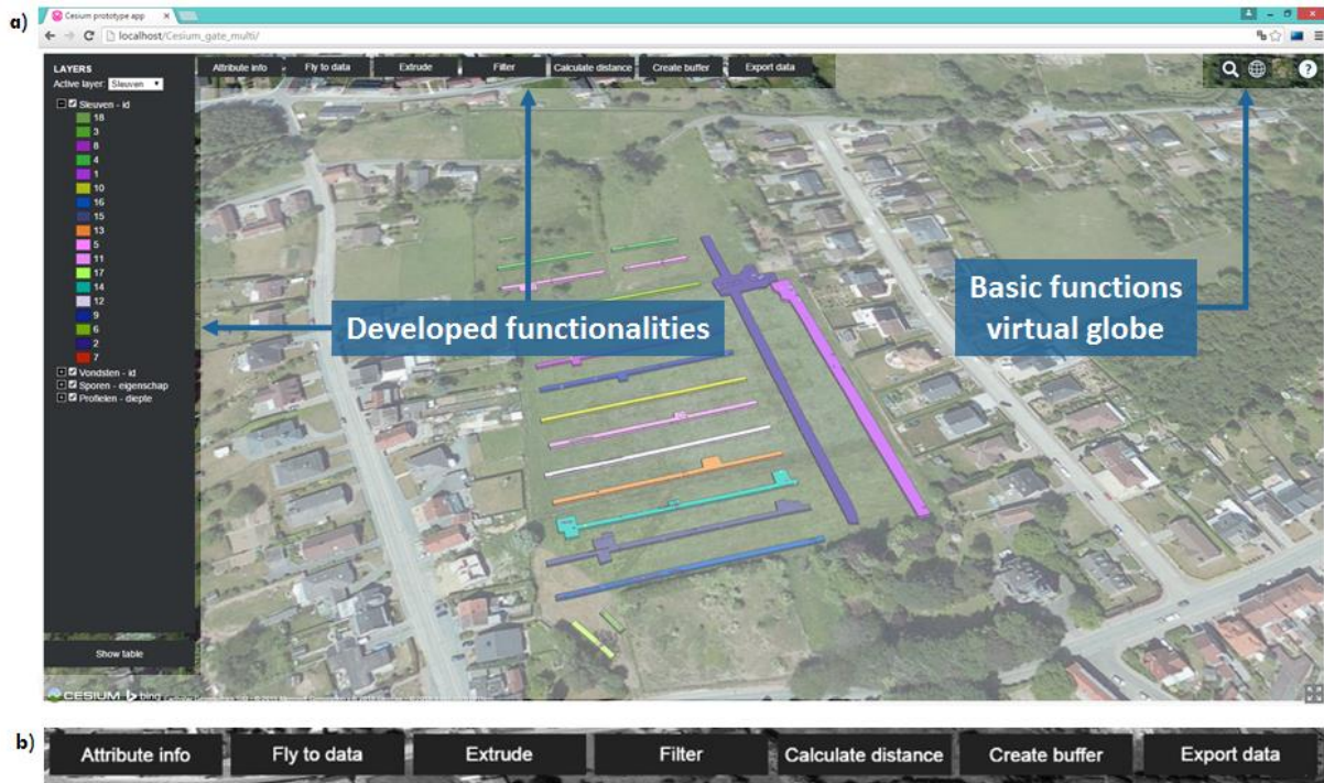
Figure 6-2 a) User interface of the prototype application, with b) zoom on top toolbar
