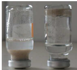
Figure 2.2. Methane oxidation led to a immobilization of the sand particles, suggesting the formation of EPS during growth. The immobilization is visualized by turning the serum vials upside down. The sand pellet remained on the bottom of the serum vial in cultures demonstrating methane oxidation, whereas the sand moved towards the other side in control samples.
