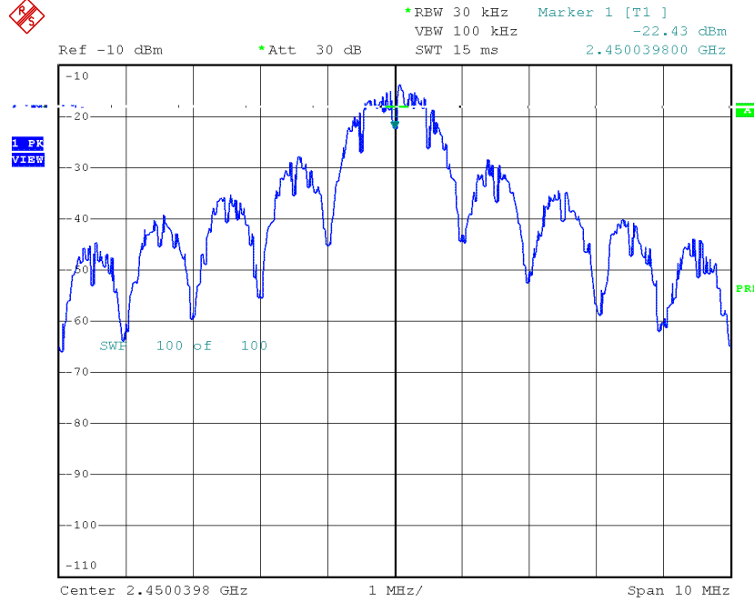
Figure 2.29: The spectral output of the generated IEEE 802.15.4 signal fulfills the absolute and relative PSD requirements.
