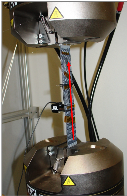
Figure 3-6. Experimental tensile test set up for measuring the local strains in the composite inner layers using FBGs.
