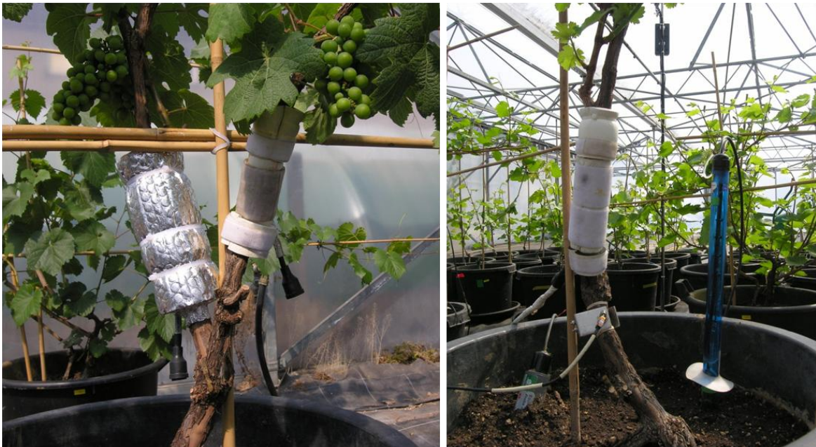
Fig. 2.11 Installation of Dynagage sensors (accuracy \pm 10\% ) (van Bavel and van Bavel, 1990) to measure sap flow rate in grapevines. These heat balance sensors calculate sap flow rate based on thermodynamics. A controlled, continuous amount of heat is applied to the exterior of the stem. The amount of heat that dissipates in radial and axial direction (by conduction) is measured. The remaining heat transported with the ascending sap (by convection) is calculated to deduce sap flow rate. The higher the convection, the higher the sap flow rate in the plant.
