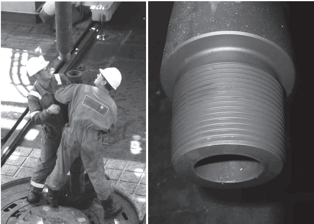
Figure 1.1: Drill pipe threaded connection
