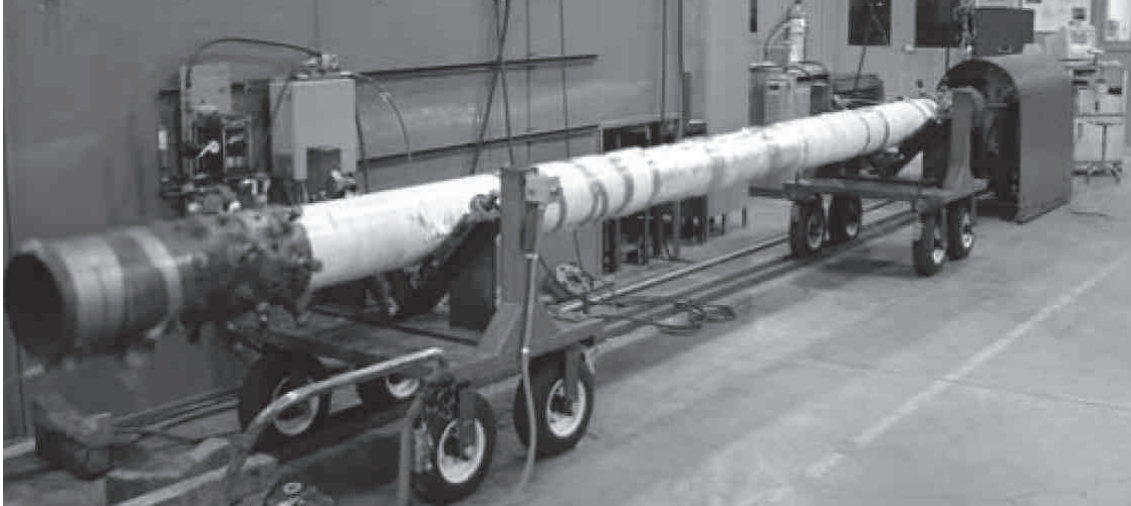
Figure 2.20: Resonant bending fatigue setup [2.95].
