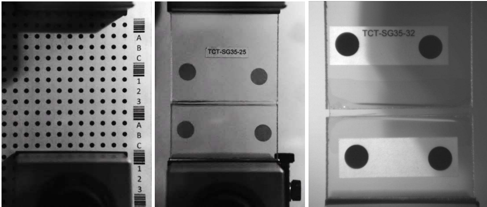
Figure V.6 – Frames used for optical measurements (from left to right) : a) calibration grid with 5 mm interspaced dots, b) first markers layout, c) second markers layout
