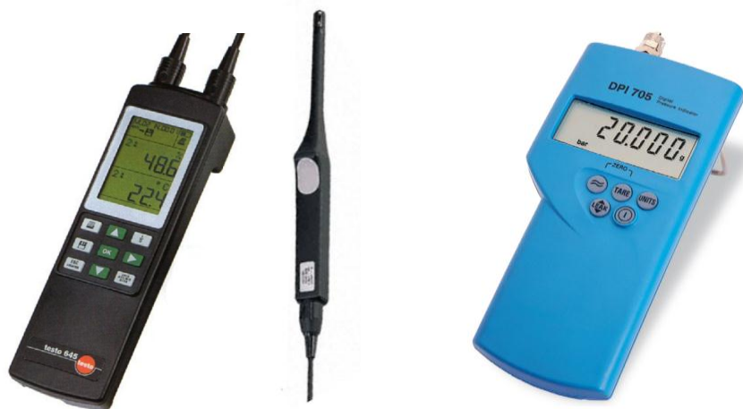
Figure 5.2 Testo 445 climate measurement device with temperature/humidity probe (left) and Digital Pressure Indicator 750 (right).
