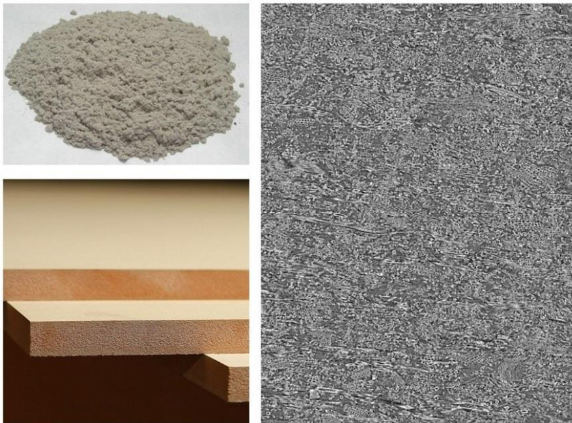
Fig 1.5. Fibers, MDF and internal microstructure of MDF (obtained with X-ray CT scanning).
