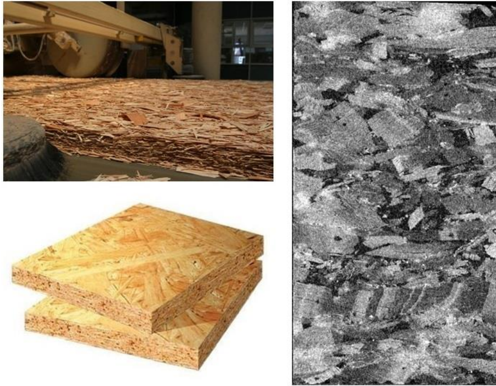
Fig 1.3. The image of flakes, OSB and internal microstructure of OSB (obtained by X-ray CT scanning).
