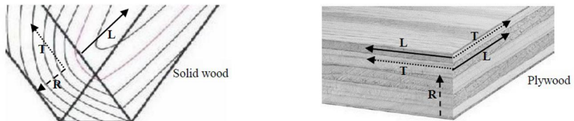
Fig 2.2. Schematic overview of directions in solid wood and plywood. L = longitudinal direction, T = tangential direction, R = radial direction.
