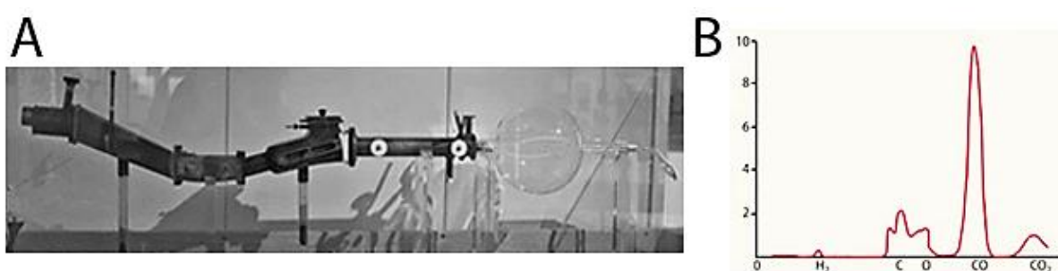
Figure 3: A) Picture of an early mass spectrometer as developed by Aston. B) One of the first mass spectra (of carbon monoxide) by Thomson [11].
