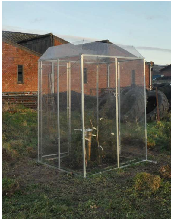
Fig. 6-2. Picture of the open top chamber at Belgium low elevation.
