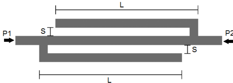
Figure 3.8: Example 3.3.2. Geometry of the double folded stub microstrip bandstop filter.
