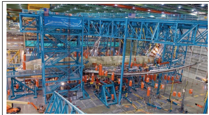
Figure 1-4: Static load test on the composite wing box (courtesy of Boeing).
