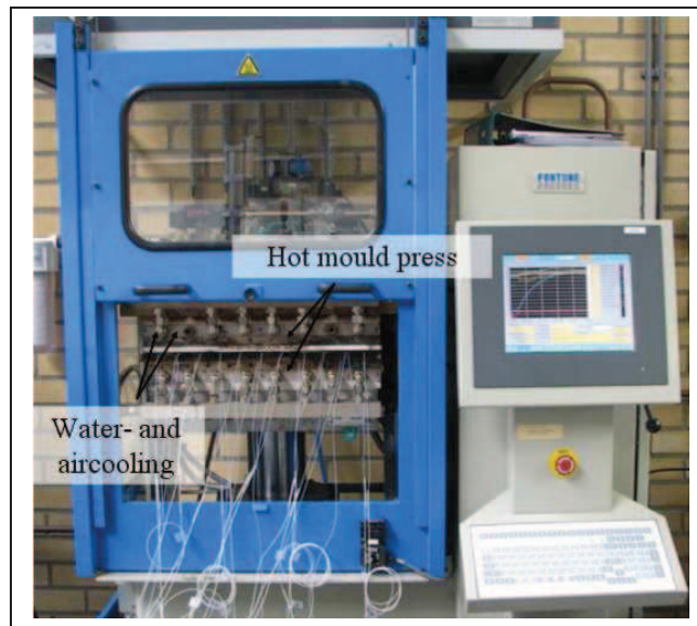
Figure 6-22: The hot mould press system of Tencate Advanced Composites, Nijverdal, the Netherlands.
