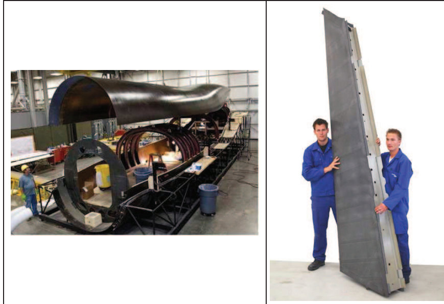
Figure 1-8: Examples of FRP structures: Fuselage with large CFRP hulls of an Advanced Composite Cargo Aircraft (left, Courtesy of U.S. Air Force Research Laboratory's ), G650 rudder with welded components made of carbon-PPS woven fabrics [9] (right).
