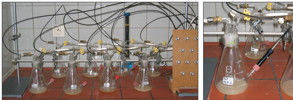
Figure 3.2. Dynamic headspace sampling of 50-ml B. cereus surface cultures (left-hand side) and SPME-extraction through a septum-sealed side inlet (right-hand side)
