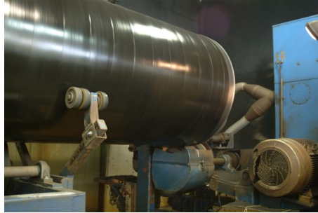
Figure 1.7: Fusion bonded epoxy (FBE) coating [1.16].
