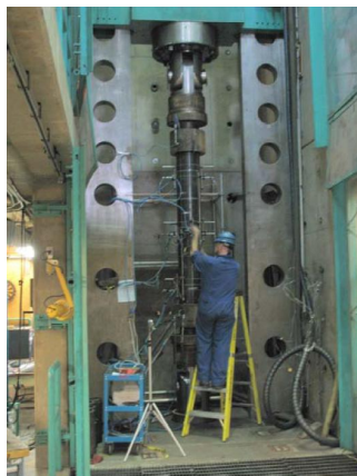
Figure 2.10: 15 MN load frame of C-FER Technologies [2.65].
